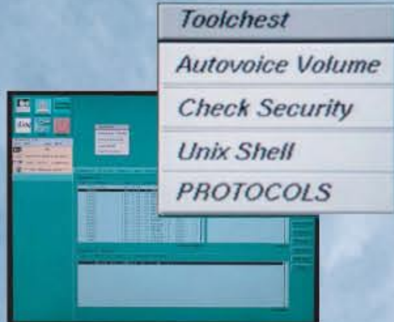
Figure 4: The "PROTOCOLS" button. The button launches the Adobe Acrobat application and opens the navigation pdf file, presenting the technologist with the home page.
